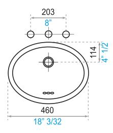
\*dimensions are in inches \*dimensions are in millimeters
